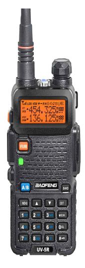
On/Off/Volume Control: Knob located on top of unit next to antenna.
